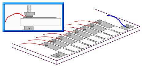
will be used for the left screw while for the rest use the washers connected to the wires as shown in the image.
